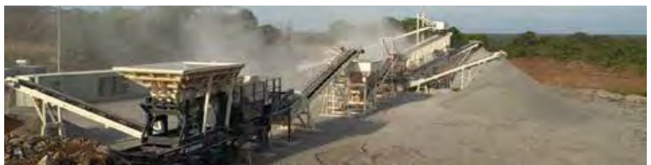
Consulmet Equipment's Second Terex MPS Aggregate Crushing Plant in Angola Terex MPS WJ3042i Wheeled Jaw Crusher with 9m3 'wing folding hopper' and Vibrating Grizzly Feeder
